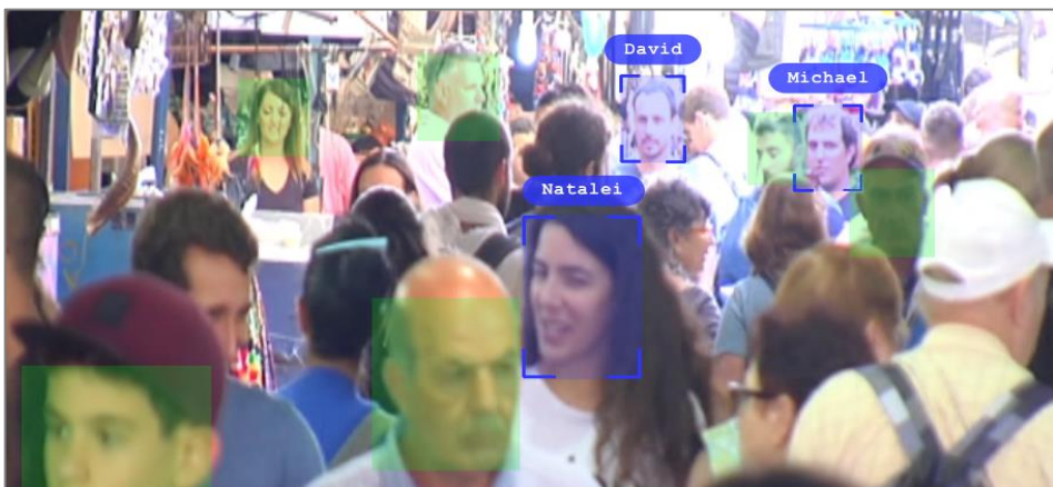
CymbloT's real-time facial recognition operates within a video surveillance camera. The green overlay shows face detection; the blue overlay signifies face recognition of persons in the target DB.
